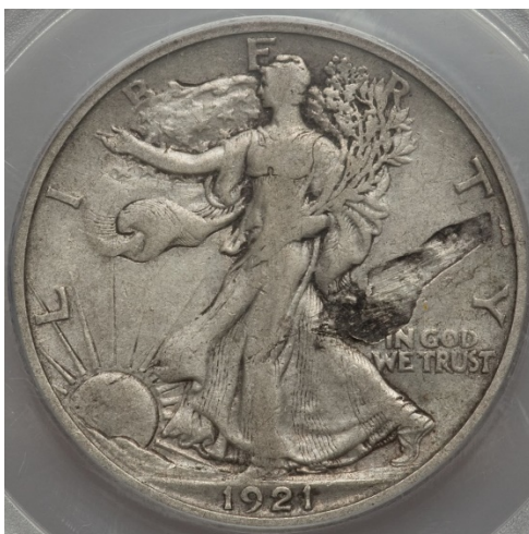
1921-S Walking Liberty half dollar, planchet lamination on obverse. Lamination errors are often the result of an improper mixture of coinage metals (reverse not affected).
