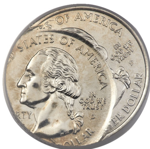
2007-D Idaho statehood quarter double-struck ( not a doubled die). The first strike was centered properly, but the accidental second strike was struck about 40 percent off-center.
