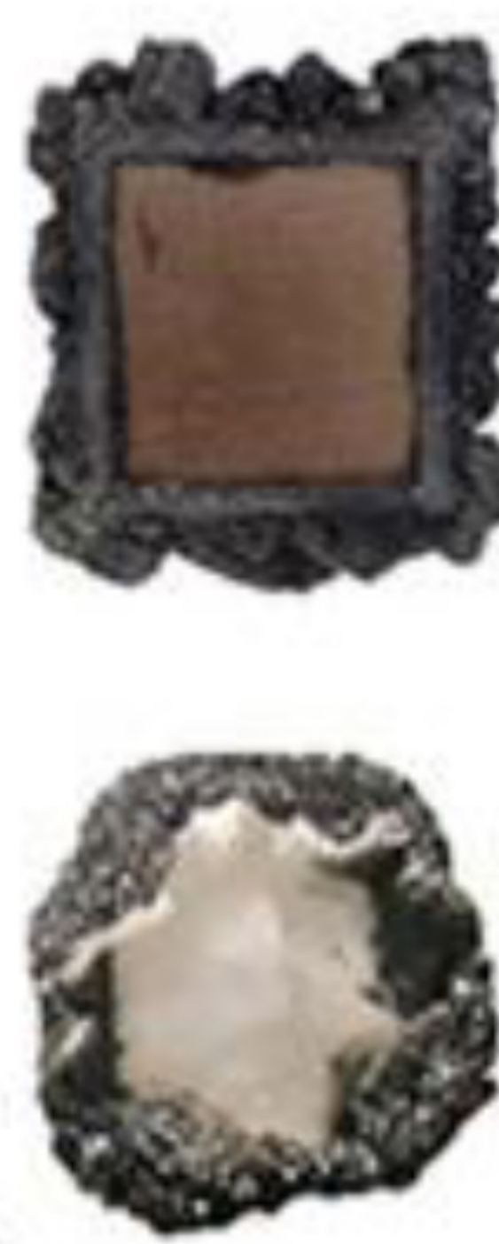
CVD crystals exhibit a flat tabular shape and a dark edge of graphite
