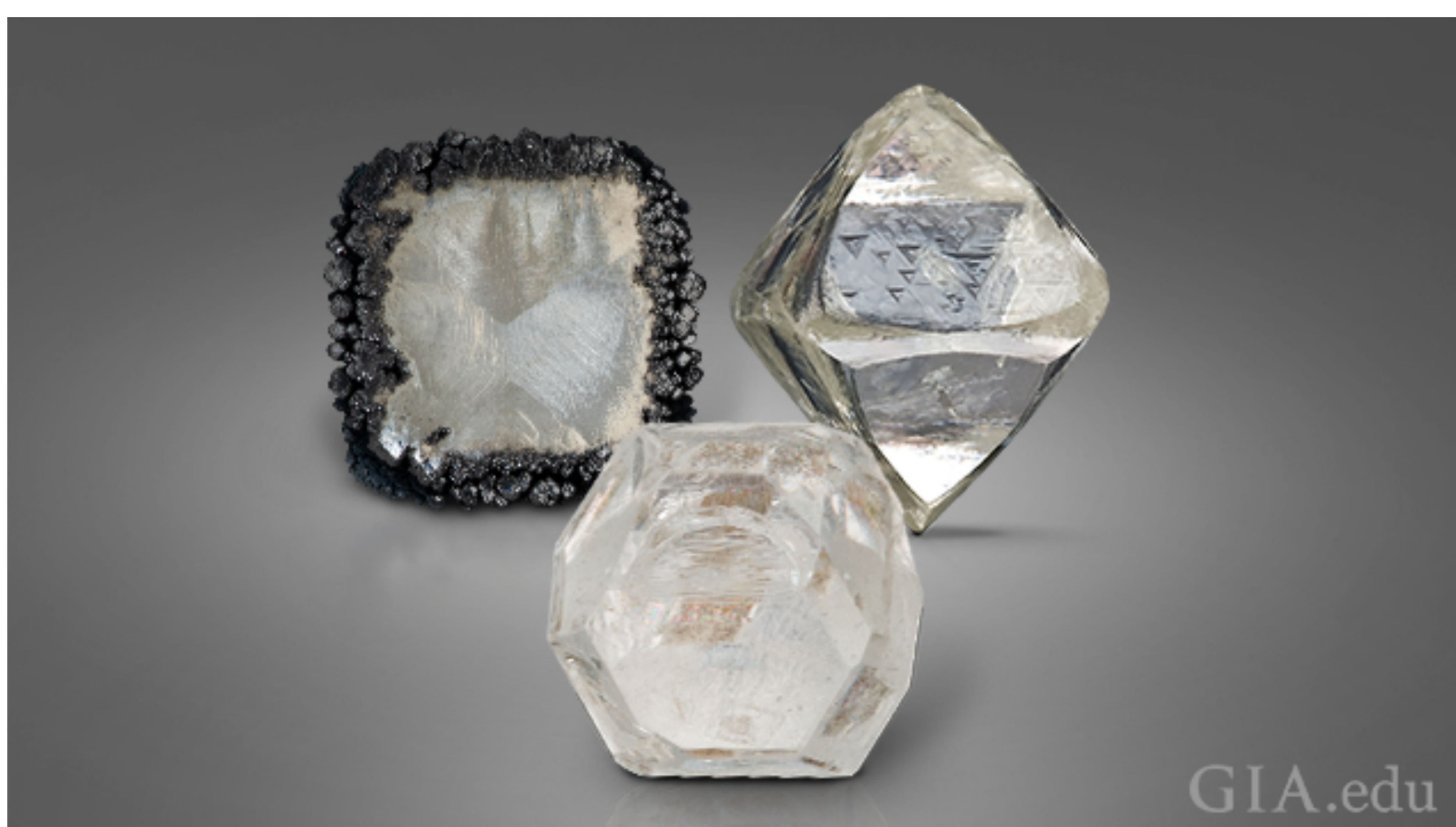
Laboratory-grown CVD rough diamond (left), laboratory-grown HPHT rough diamond (middle) and natural rough diamond (right)
